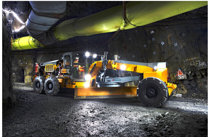
Fig. 1: MacLean Engineering GR5 grader is a purpose-built machine for road surface maintenance in mining applications. The vehicle can be steered both by turning the front-axle wheels as well as by hydraulically actuating the angle of an articulation joint that connects the front and rear components of the machine [Photo source: macleaneengineering.com].
